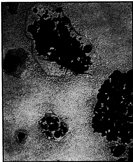
FIG. 1. Tetra copper calcium oxychloride evaporated under electron bombardment and redeposited over the supporting film ( \times 50,000 ).
